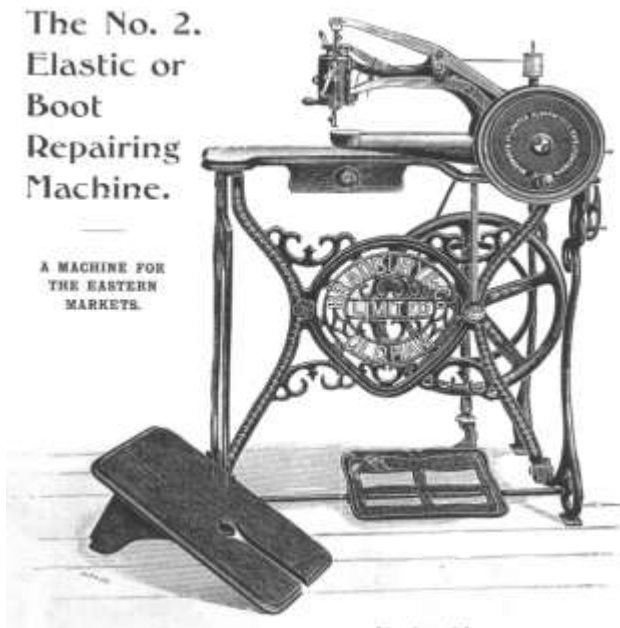
Figure 4: No.2 Elastic machine -note the size of the Arm
